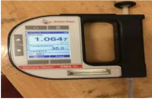
Figure 4. Density Measurement of Nanofluid Figure 5. Specific Heat Measuring Apparatus
