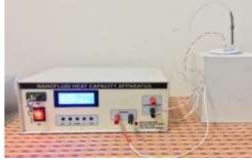
Figure 4. Density Measurement of Nanofluid Figure 5. Specific Heat Measuring Apparatus
