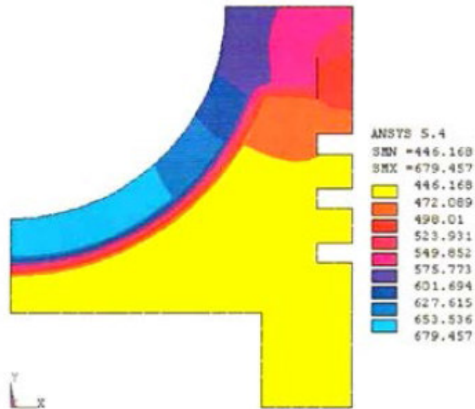
Figure 3: Temperature distribution in the air-gap piston with crown made up of the Al-alloy.
