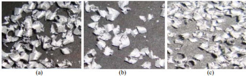
Figure 2: Size of chips during machining of as cast AA2024/SiCp MMCs reinforced with (a) 10 wt % SiCp, (b) 12.5 wt % SiCp and (c) 15 wt % SiCp.
