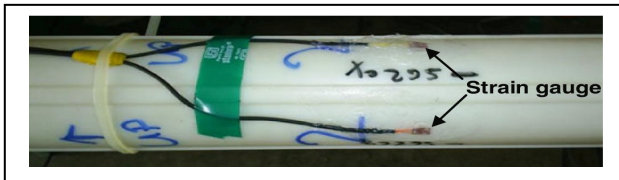
Fig. 3 Strain gauges fixed on inclinometer casing
