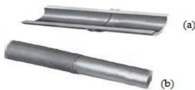
Figure 15: Cut-section of friction welded AA1100 alloy and 316 stainless steel (a) weld joint with flash removed (b).
