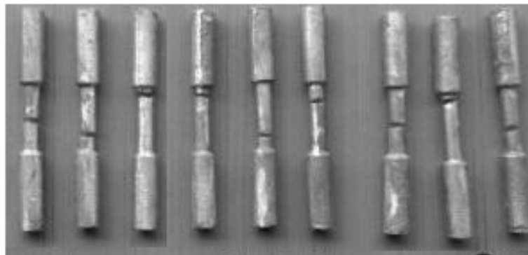
Figure 4: Tested tensile specimens.
