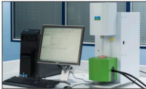
Figure 2: TMA analyzer for the measurement of thermal expansion of investment shell moulds.
