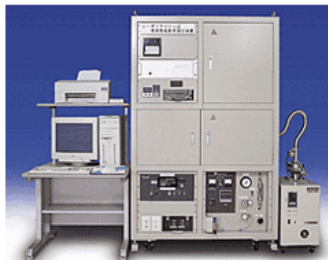
Figure 4: Laser flash method for the measurement of thermal conductivity of investment shell moulds.
