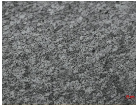
Figure 3: Microstructure of AA2219 alloy used for turbine impeller.
