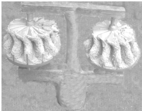
Figure 1: Cast turbine impeller in investment shell moulds.
