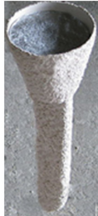
Figure 1: Hypoeutectic Al-Si alloy cast in Boron coated investment shell mould.
