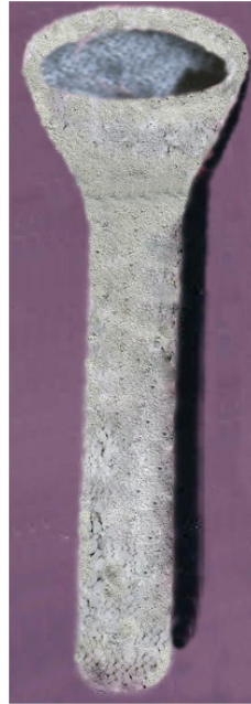
Figure 1: Hypoeutectic Al-Si alloy cast in Strontium coated Titania investment shell mould.
