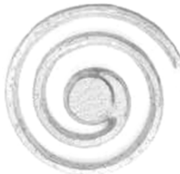
Figure 2: Fluidity spiral of Elektron 21 alloy.
