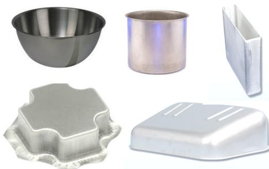
Figure 2: Different shapes fabricated by conventional deep drawing process
