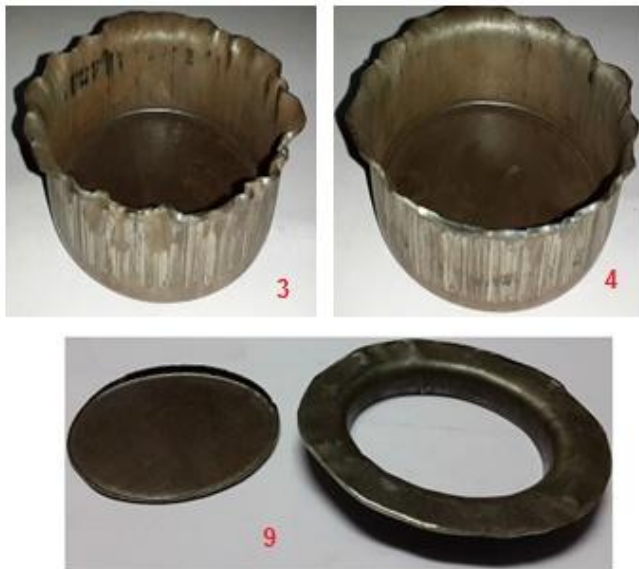
Figure 19: Experimental validation of deep drawing nickel 201
