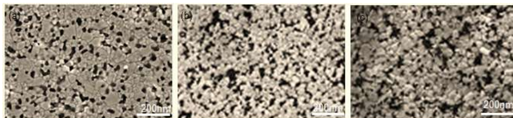
Figure 4: Microstructures of Al/ZrO 2 composites: (a) 30 vol.% pure ZrO 2 (b) 30 vol.% ZrO 2 doped with 8% Y 2 O 3 and (c) 30 vol.% ZrO 2 doped with 15% Y 2 O 3 .
