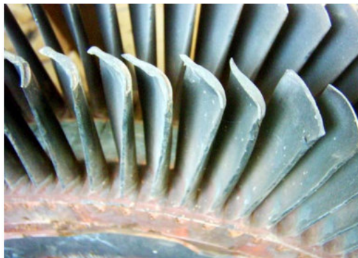
Figure 1: Blades operated at high temperature.
