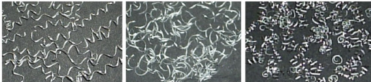
Figure 1: Chips formed during machining of Al/SiCp metal matrix composites.
