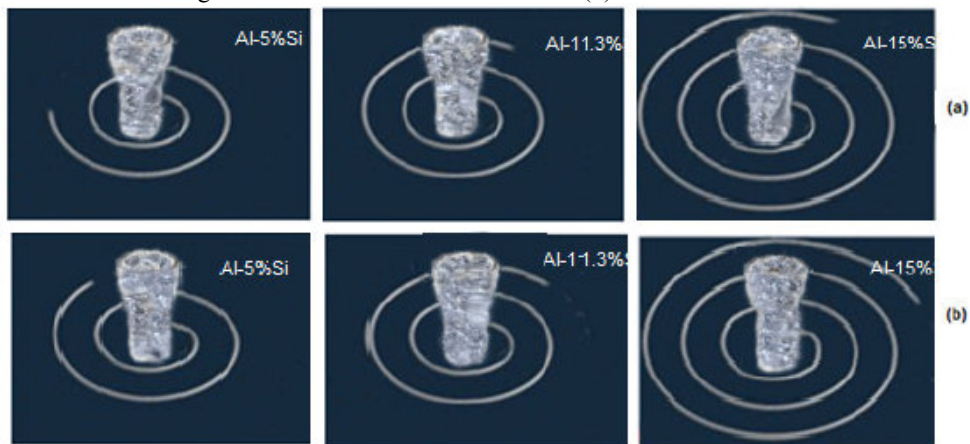
Figure 6: Fluid spirals cast in (a) modified and (b) unmodified Al-Si alloys.
