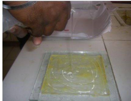
Fig 3.4. Applying PVA to the mould
