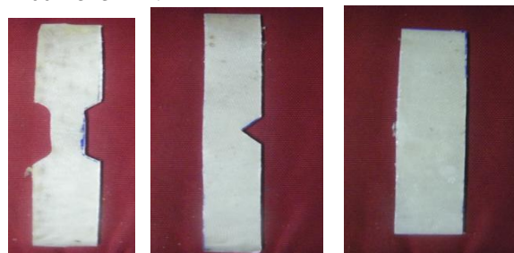
Fig: 3.14. Specimen for Tensile, Impact, Flexural tests
