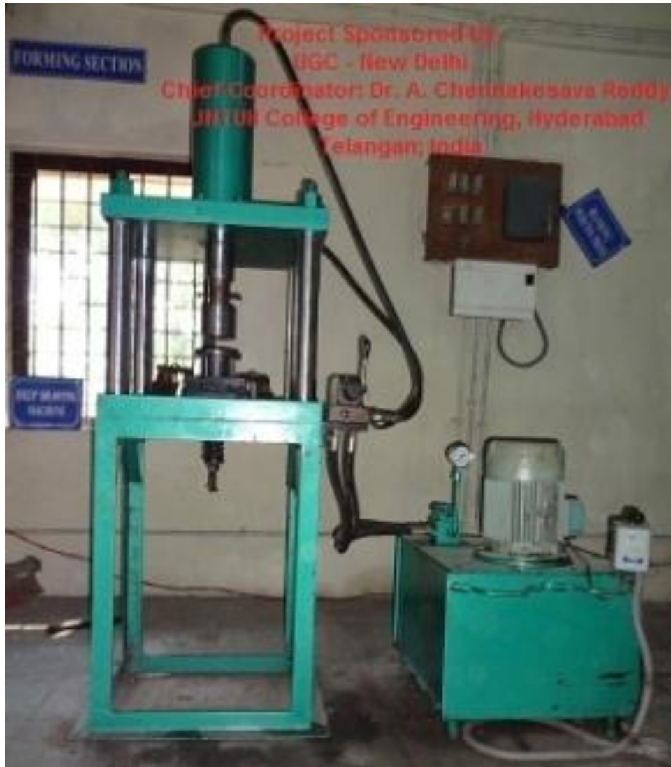
Figure 1: Hydraulic type deep drawing press.
