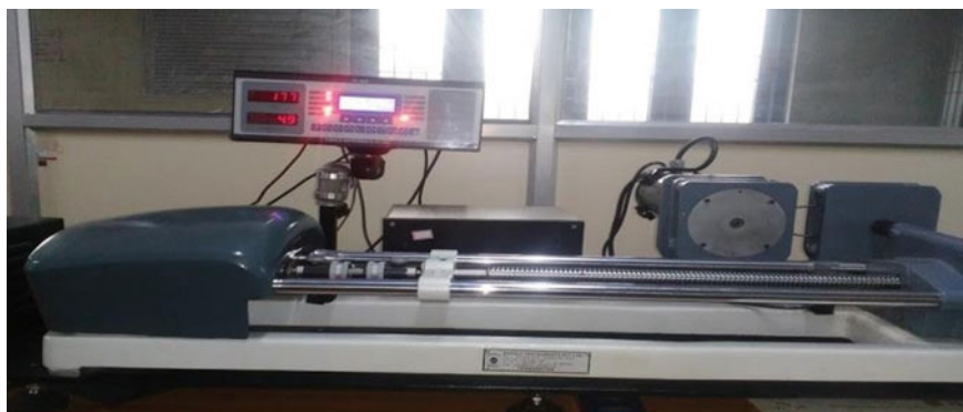
Fig. 47.1 Tensometer for testing the specimens
