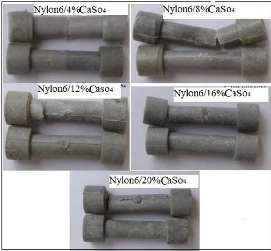
Fig. 47.2 Tensile specimens of Nylon/CaSO 4
