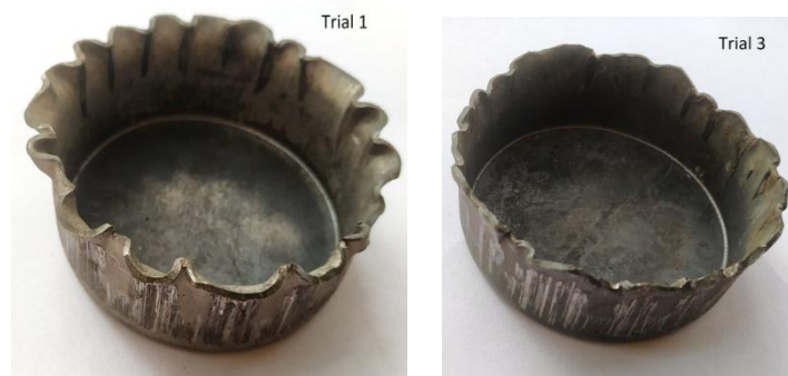
Figure 12: The successful deep drawn cup
