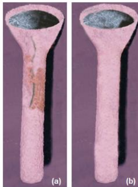
Figure 6: Thermal shock in the investment shell moulds made of (a) \alpha -cristobalite (b) \beta -cristobalite filler material.
