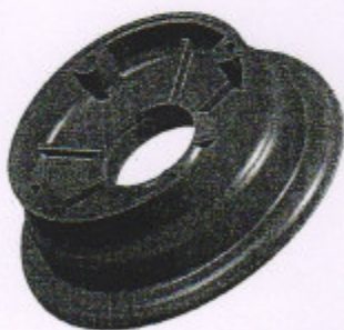
Fig 1. Three- Dimensional Model of Nose Wheel Half Hub Casting
