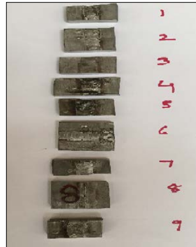
Fig. 4: Nine welded specimen for Hardness test and microstructure analysis.
