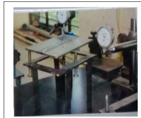
Fig. 1: Stand set up of angular distortion test
