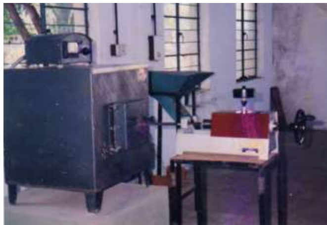
Figure 2. Hot bending strength test of investment shells.
