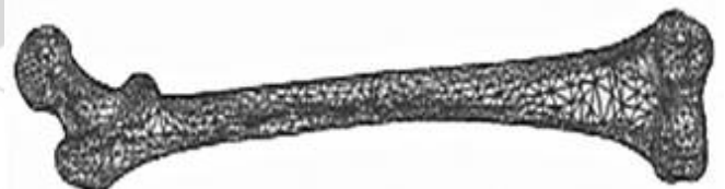
Figure 5: Finite modeling of femur bone
