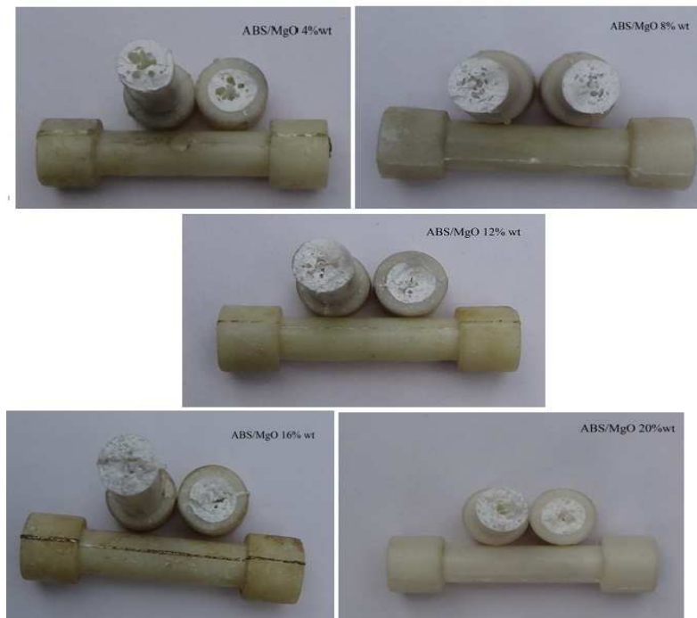
Figure 1: Tensile Specimens of ABS/MgO.
