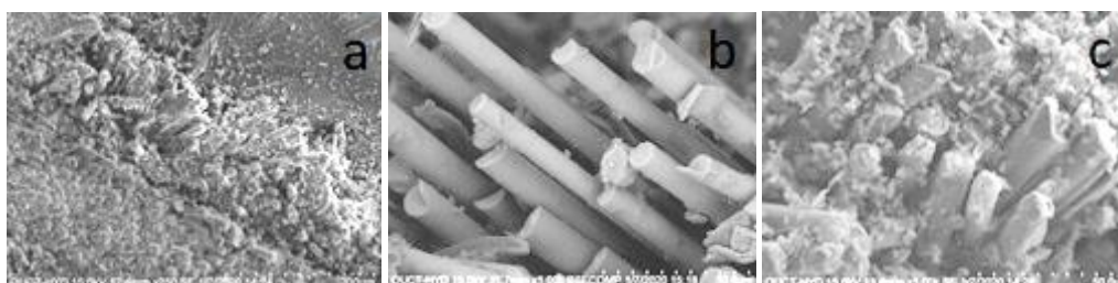
Fig.7. SEM images of samples subjected to Flexural strength (a,b,c sample sides)
