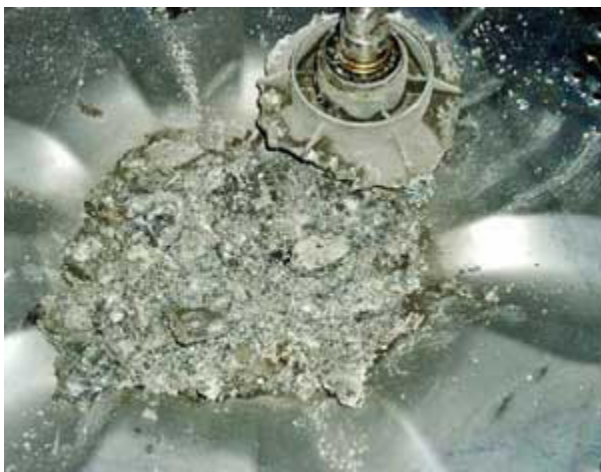
Figure 1. Corrosion of Al products.
