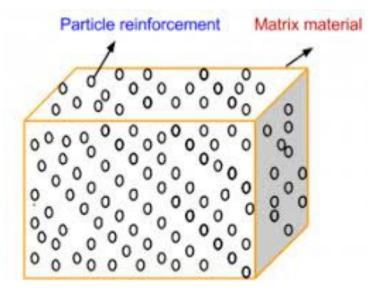
Particulate composites offer several advantages. They provide reinforcement to the matrix material thereby strengthening the material. The combination of reinforcement and matrix can provide for very specific material properties. For example, the inclusion of conductive reinforcements in a plastic can produce plastics that are somewhat conductive. Particulate composites can often use more traditional manufacturing methods such as injection molding which reduces cost.
