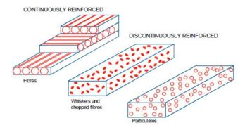
Continuous reinforcement uses monofilament wires or fibers such as carbon fiber or silicon carbide. Because the fibers are embedded into the matrix in a certain direction, the result is an anisotropic structure in which the alignment of the material affects its strength. One of the first MMCs used boron filament as reinforcement. Discontinuous reinforcement uses "whiskers", short fibers, or particles. The most common reinforcing materials in this category are alumina and silicon carbide.
