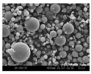
Aluminum Oxide ( $Al_2O_3$ ). Aluminum oxide (alumina) is the workhorse of advanced technical ceramics. It has good mechanical and electrical properties, wear resistance and corrosion resistance. It has relatively poor thermal shock resistance. It is used as an electrical insulator for a number of electrical and electronic applications, including spark plug insulators and electronic substrates. It is also used in chemical, medical and wear applications.
