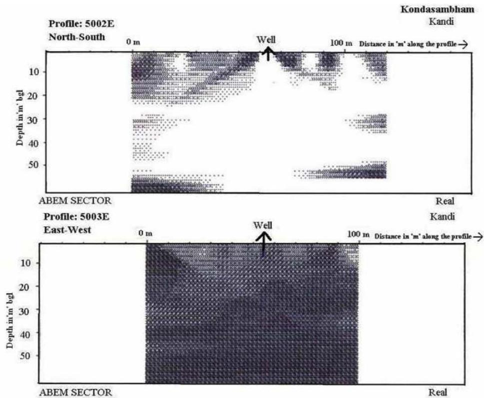
Fig.4. Vertical cross section of VLF Electromagnetic data of a successful well at the Kondasambham village.
