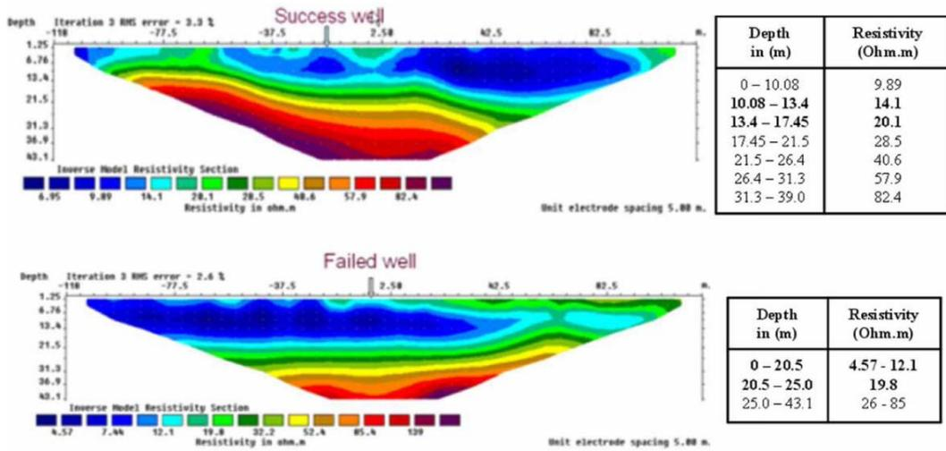
Fig.7. Electrical Resistivity images at Successful and Failed Wells near the road of Sivaram village.
