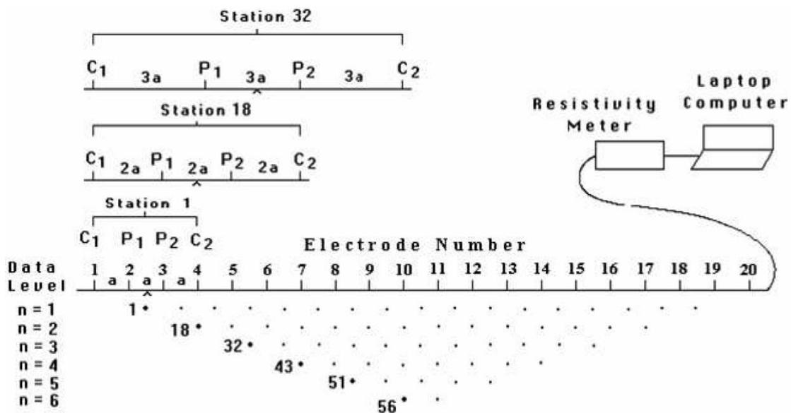
Fig.6. Sequence of measurements in resistivity imaging to build up a pseudosection
