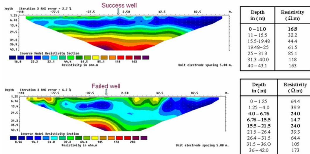
Fig.9. Electrical Resistivity images at Successful and Failed Wells at the Kondasambham Village.
