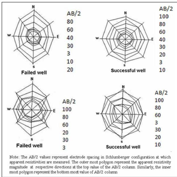
Fig.5. Apparent resistivity polygons of the wells at the Sivaram village
