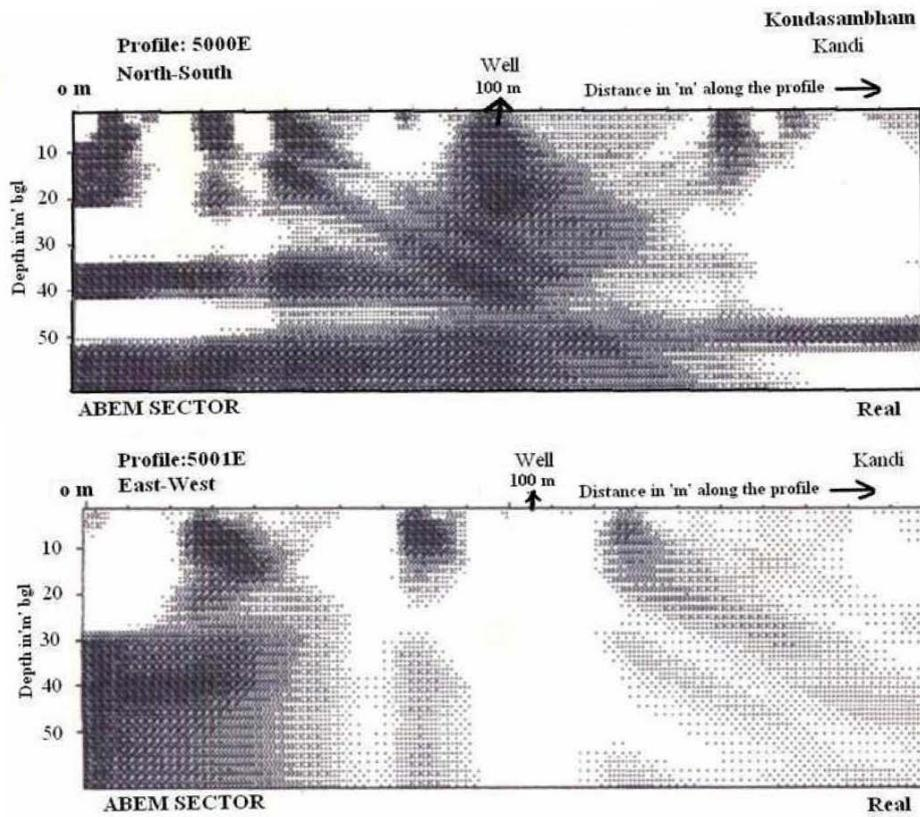
Fig.3. Vertical cross section of VLF Electromagnetic data of a failed well at the Kondasambham village.
