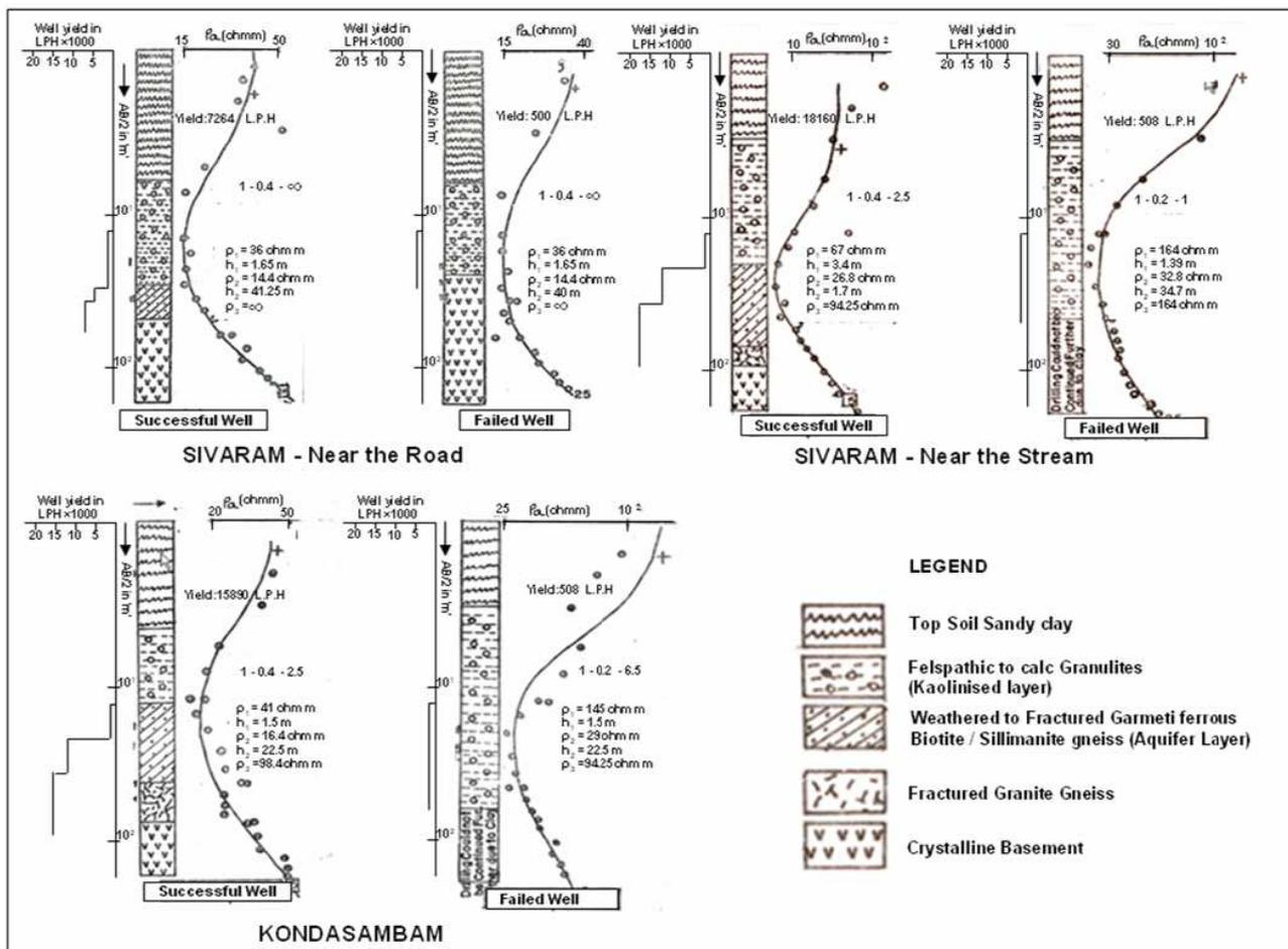
**Fig.2.** Vertical electrical sounding curves, yield logs and lithologs of adjacent success and failed Wells near the road at Sivaram village, near the stream at Sivaram village and at Kondasambham Village.
