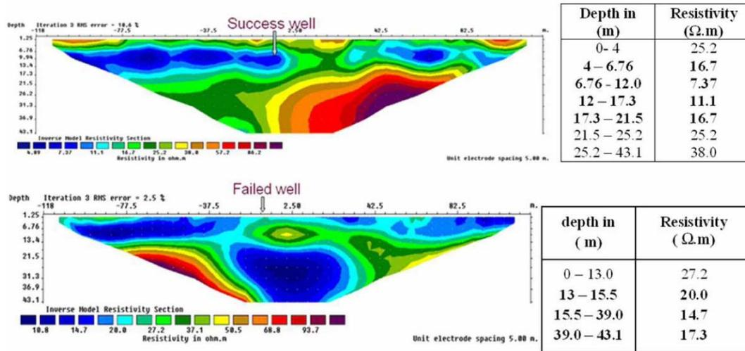
Fig.8. Electrical Resistivity images at Successful and Failed Wells near the stream of Sivaram village.
