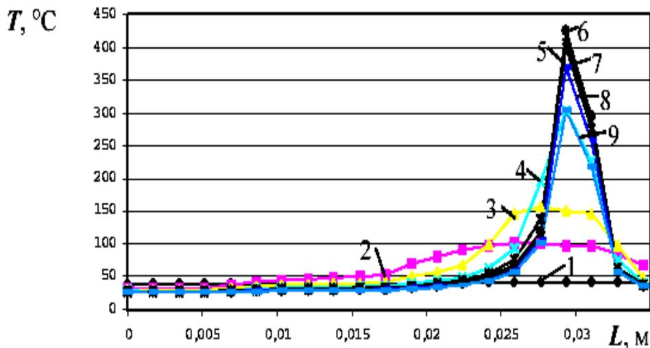
Fig. 4 Distribution of temperature across lining width at various braking time.
