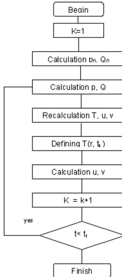
Fig.2 Flowchart for solving thermoelastic contact problem
