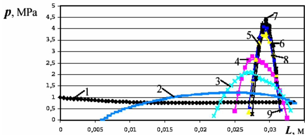
Fig. 3 Distribution of contact pressure across lining width at various braking times.
