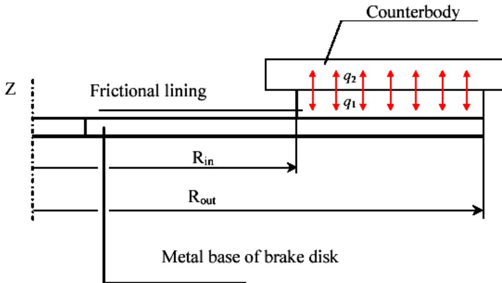
Fig.1 Schematic representation frictional contact model
