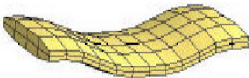
Fig.1 Finite element mesh of a yarn segment
