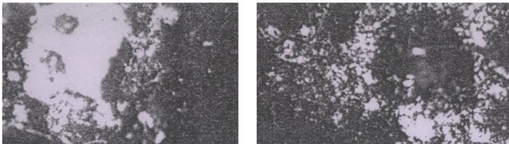
Figure 8: Micrographs showing different types of craters: (a) Al-10% SiC MMC, electrode Br (-), Current: 10A, Pulse duration:192 $\mu$ s (b) Al-10% SiC MMC, electrode Br (-), Current: 10A, Pulse duration:425 $\mu$ s
