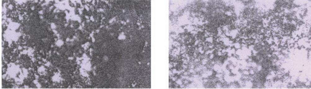
Figure 9: Micrographs showing different types of pock marks and pin marks: (a) Al-10% SiC MMC, electrode Br (-), Current: 10A, Pulse duration:192 $\mu$ s (b) Al-10% SiC MMC, electrode Br (-), Current: 10A, Pulse duration:425 $\mu$ s
