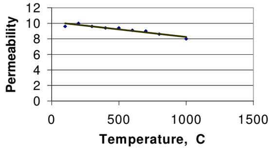
Figure 4. Effect of sintering on the permeability of the shells
