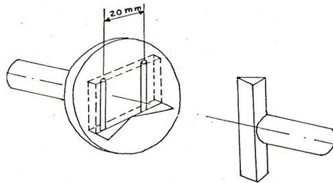
Figure 1. Hot modulus of rupture test
