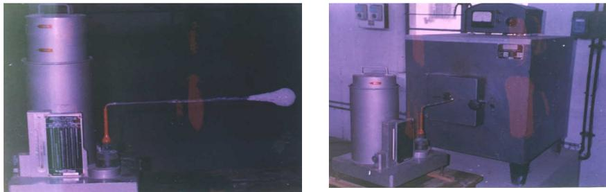
Figure 2. Hot permeability test
