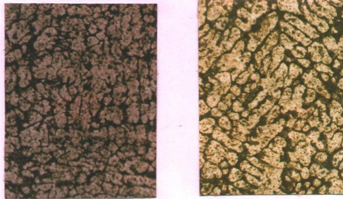
Figure 4. Micrographs of Al-Si-Mg alloy castings, 100X. (a) Casting from the fly ash shell (b) Casting from the alumina shell
