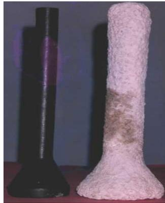
Figure 1. Wax pattern and ceramic shell
