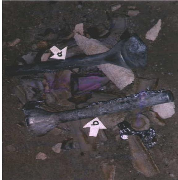
Figure 2. Castings after knocking out from the ceramic shells
