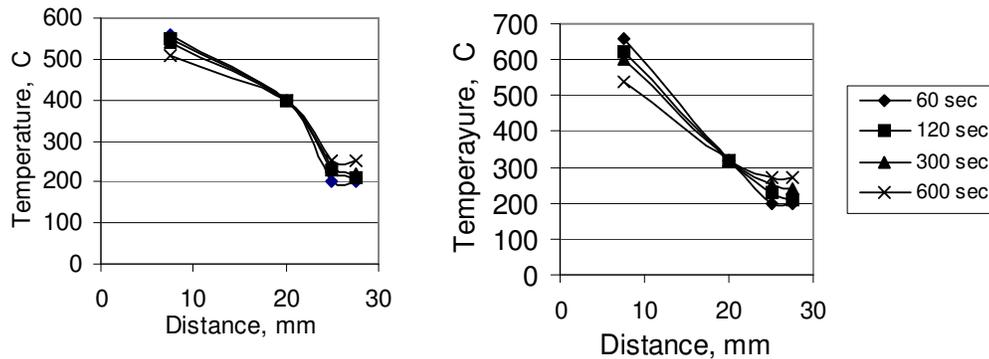
Figure 3. Cooling contours while casting in (a) the flyash shell and (b) the alumina shells.
