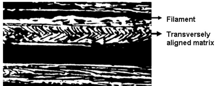
Fig.8 Scanning electron micrograph of transversely aligned matrix (10 $\mu$ m)
