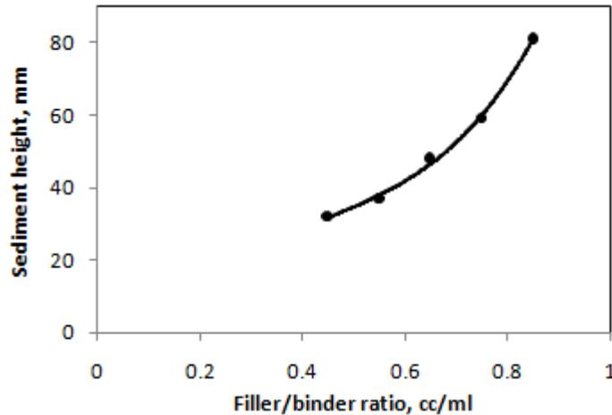
Figure 4. Effect of filler loading on sedimentation.
