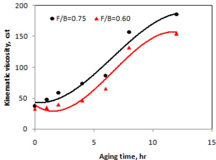
Figure 5. Effect of aging time on viscosity of ceramic slurry.
