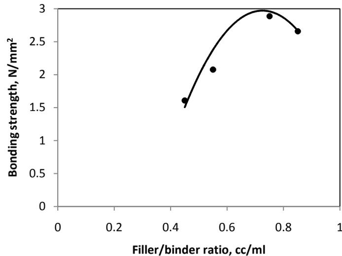
Figure 6. Effect of filler loading on shell strength.
