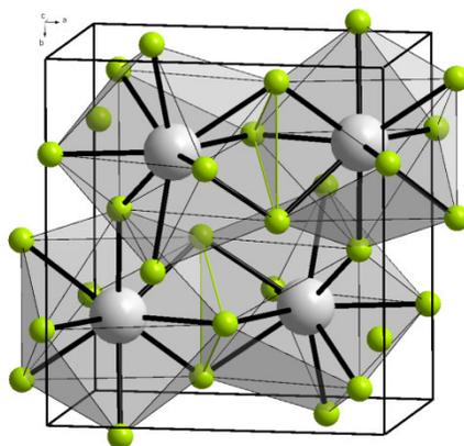
Figure 1. Crystal structure of yttria.
