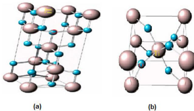
Figure 5. Crystal structure of  $TiO_2$ : (a) anatase Phase and (b) rutile Phase.
