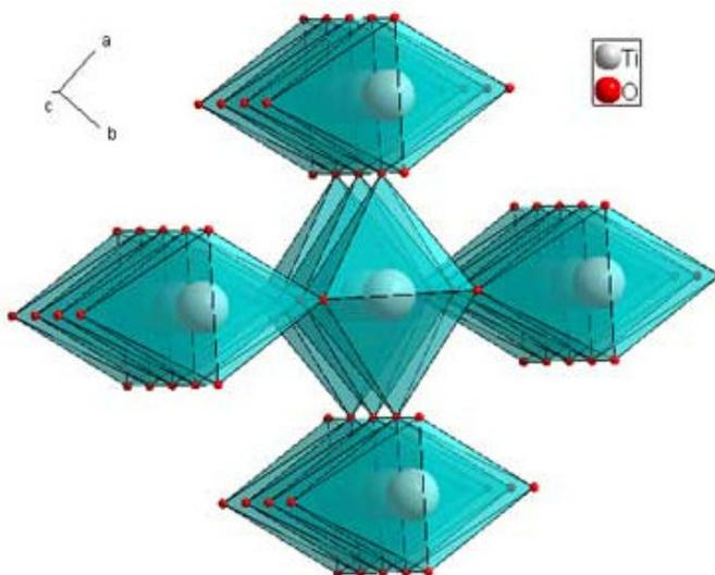
Figure 1. Crystal structure of rutile.
