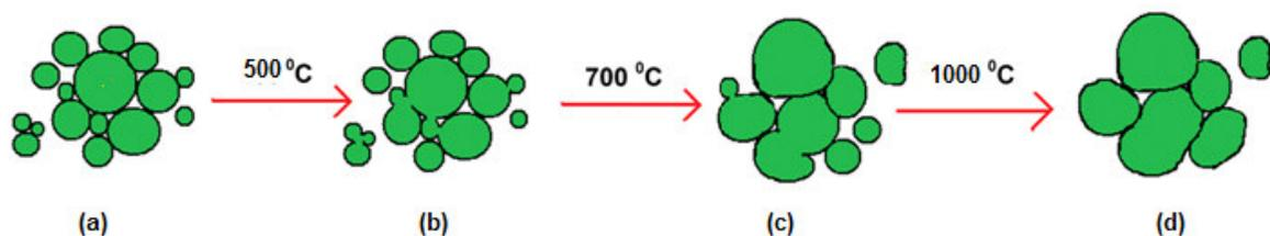
Figure 6. Schematic representation of temperature-induced grain growth of  $TiO_2$ .
