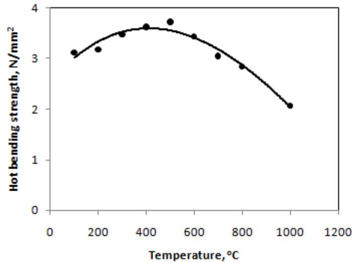
Figure 4. Effect of temperature on hot shell strength.
