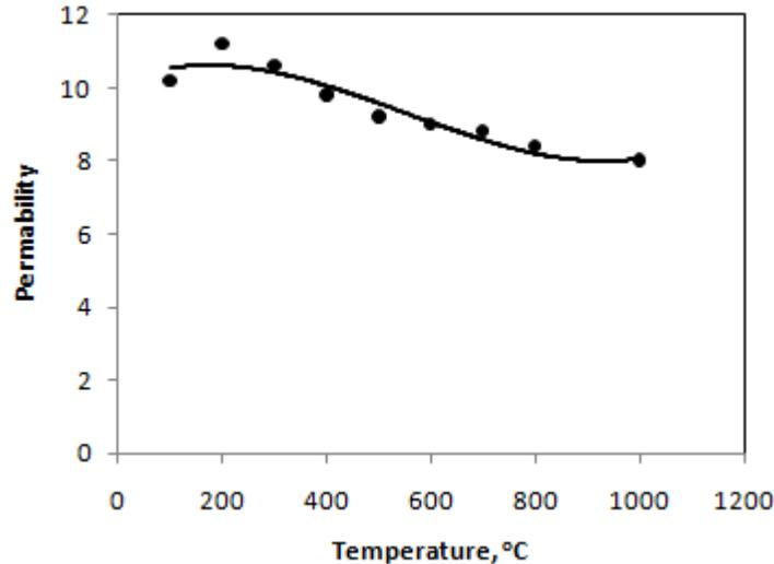
Figure 7. Effect of temperature on shell permeability.
