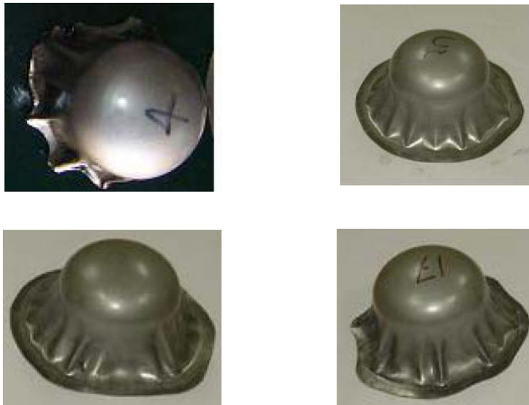
Figure 12. Wrinkling at the lip area(Zone- II) of Inconel-718 blank(Draw Ratio-2.14).
