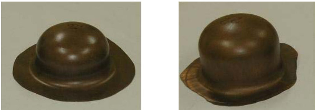
Figure 14. Defect-free hydroformed Copper blanks with draw ratio 2.14.
