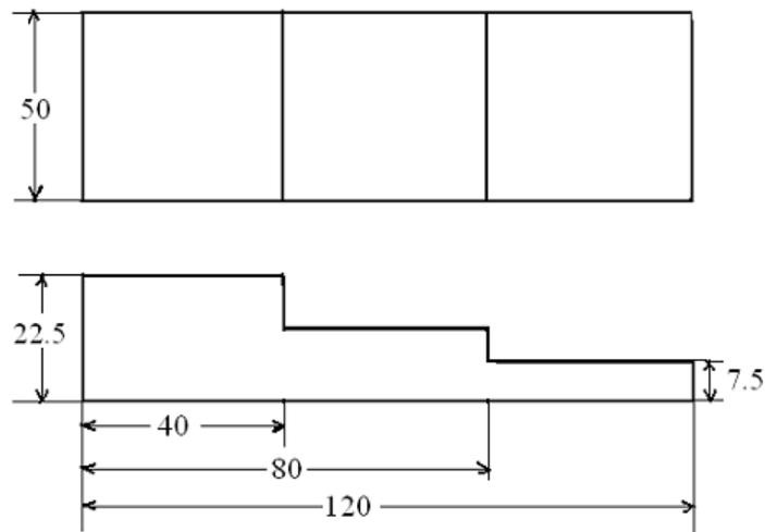
Figure 1. Casting design
