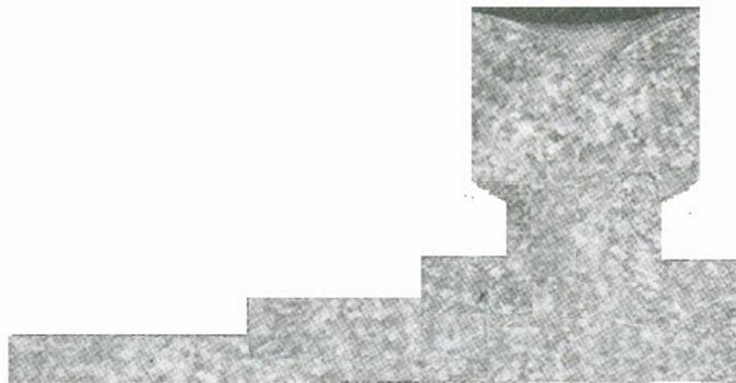
Figure 7. Gravity diecasting section having the process parameters: alloy-1, pouring temperature =  $725^{\circ}\text{C}$ , mould pre-heat temperature =  $400^{\circ}\text{C}$ , and degasified with 1.25% tetrachlorethane.
