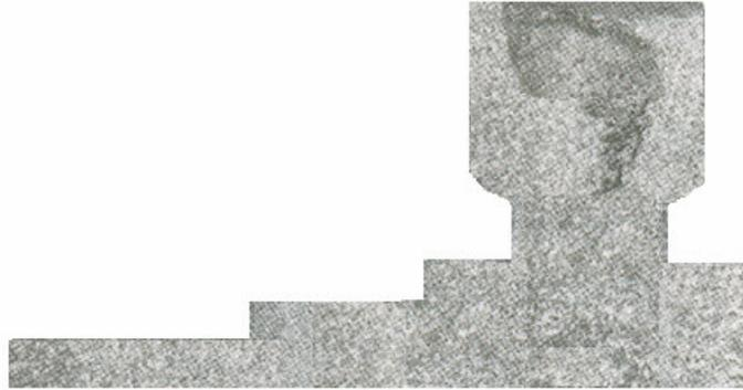
Figure 6. Gravity diecasting section having the process parameters: alloy-1, pouring temperature =  $700^{\circ}\text{C}$ , mould pre-heat temperature =  $300^{\circ}\text{C}$ , and degasified with 1.00% tetrachlorethane.
