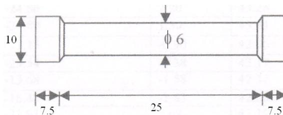
Figure 4. Tensile specimen, all dimensions are in mm
