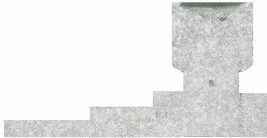
Figure 13. Gravity diecasting section having the process parameters: alloy-3, pouring temperature =  $725^{\circ}\text{C}$ , mould pre-heat temperature =  $300^{\circ}\text{C}$ , and degasified with 0.75% tetrachlorethane
