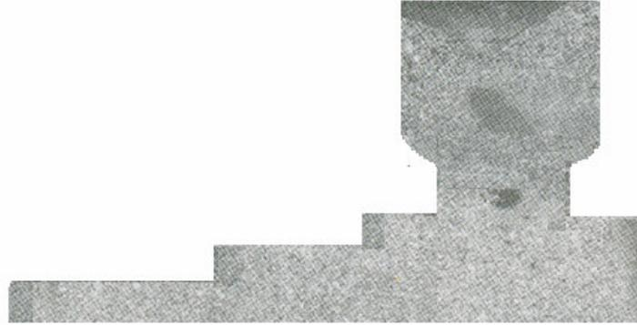
Figure 9. Gravity diecasting section having the process parameters: alloy-2, pouring temperature =  $700^{\circ}\text{C}$ , mould pre-heat temperature =  $400^{\circ}\text{C}$ , and degasified with 0.75% tetrachlorethane
