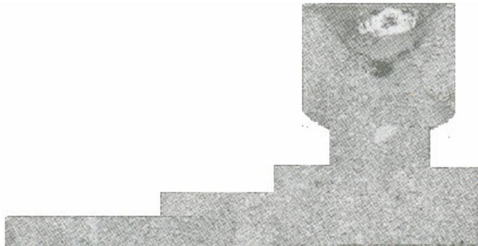
Figure 8. Gravity diecasting section having the process parameters: alloy-2, pouring temperature =  $675^{\circ}\text{C}$ , mould pre-heat temperature =  $300^{\circ}\text{C}$ , and degasified with 1.25% tetrachlorethane
