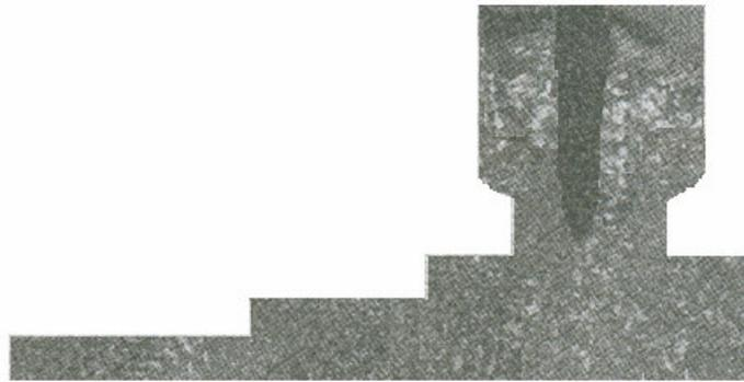
Figure 10. Gravity diecasting section having the process parameters: alloy-2, pouring temperature =  $725^{\circ}\text{C}$ , mould pre-heat temperature =  $200^{\circ}\text{C}$ , and degasified with 1.00% tetrachlorethane
