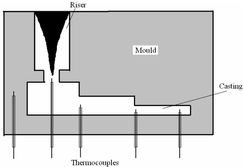
Figure 3. Setup for the measurement of solidification time
