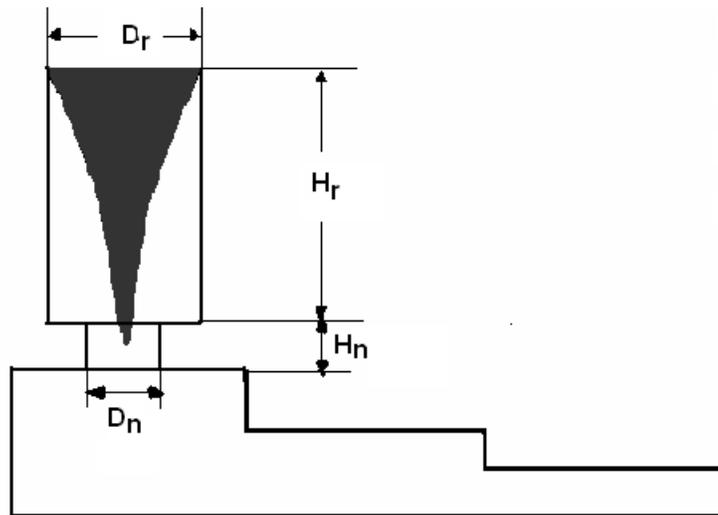
Figure 2. Location of riser on the casting
