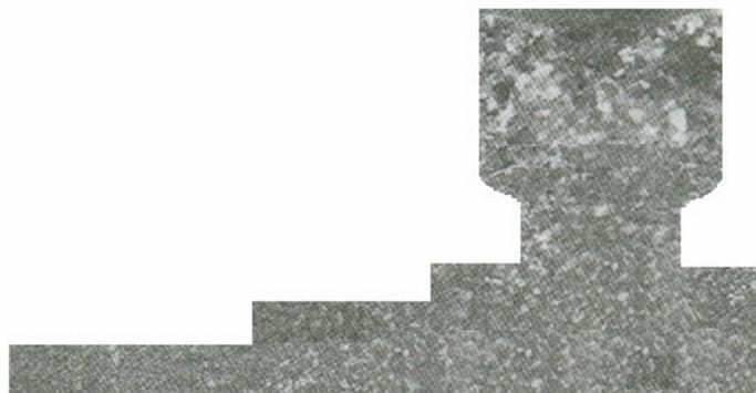
Figure 5. Gravity diecasting section having the process parameters: alloy-1, pouring temperature = 675<sup>0</sup> C, mould pre-heat temperature = 200<sup>0</sup> C, and degasified with 0.75% tetrachlorethane.
