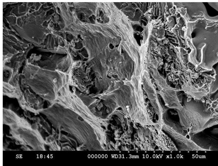
**Figure 11: SEM of fracture surface of heat treated tensile sample (SiC particle size =  $10\mu\text{m}$  and volume fraction = 20%)**
