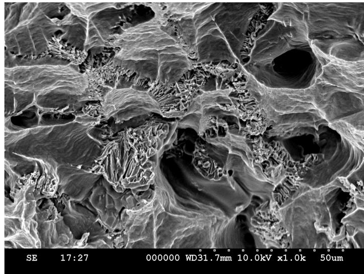
**Figure 12: SEM of fracture surface of heat treated fatigue sample (SiC particle size = 10µm and volume fraction = 20%)**
