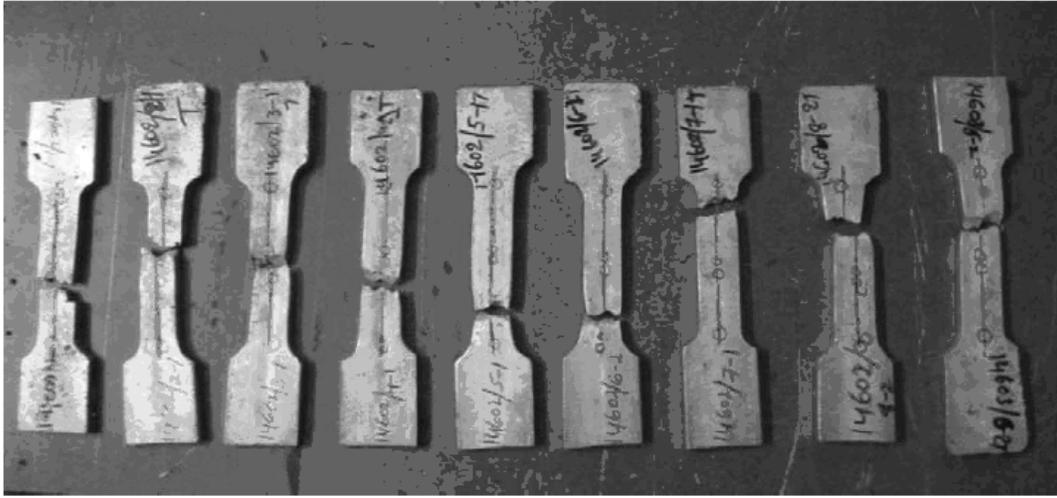
**Figure 3: Tested tensile Al/SiC Composite specimens**
