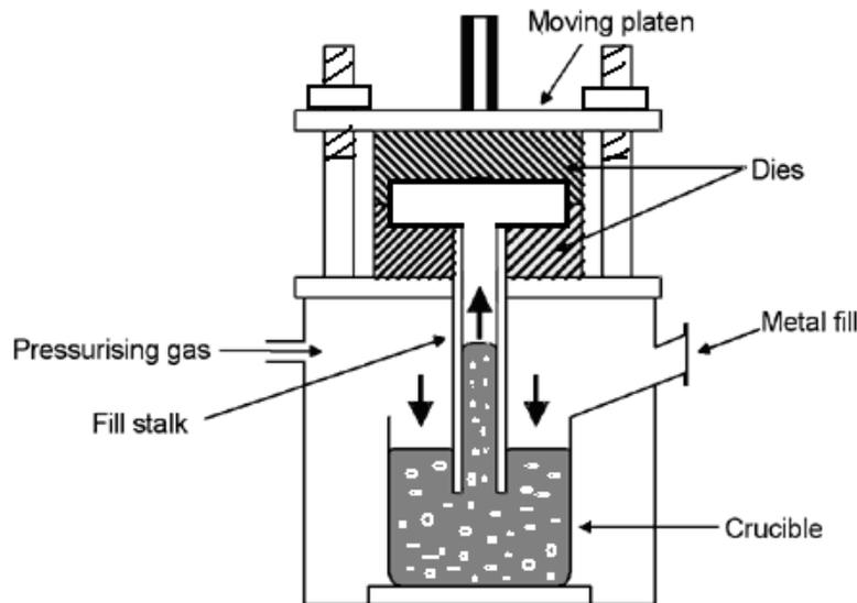
**Figure 1: Schematic representation of low pressure die casting process**
