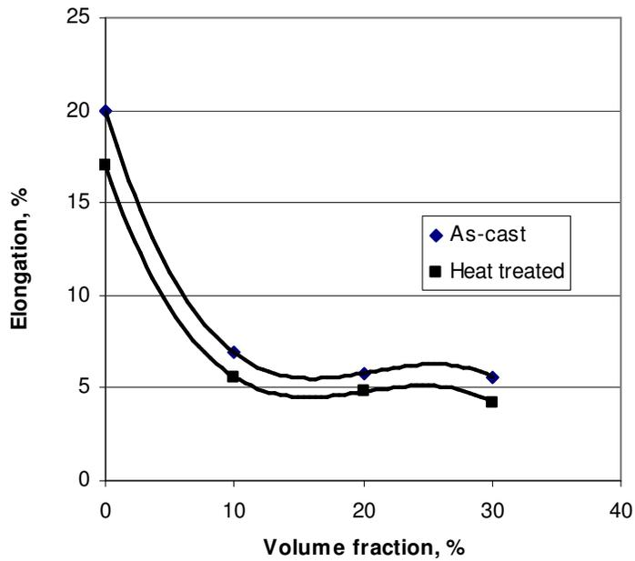
Figure 9: Variation of the ductility with the volume fraction of SiC particles
