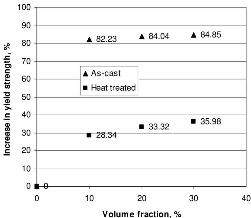
**Figure 7: Increase in yield strength due to reinforcement and heat treatment**
