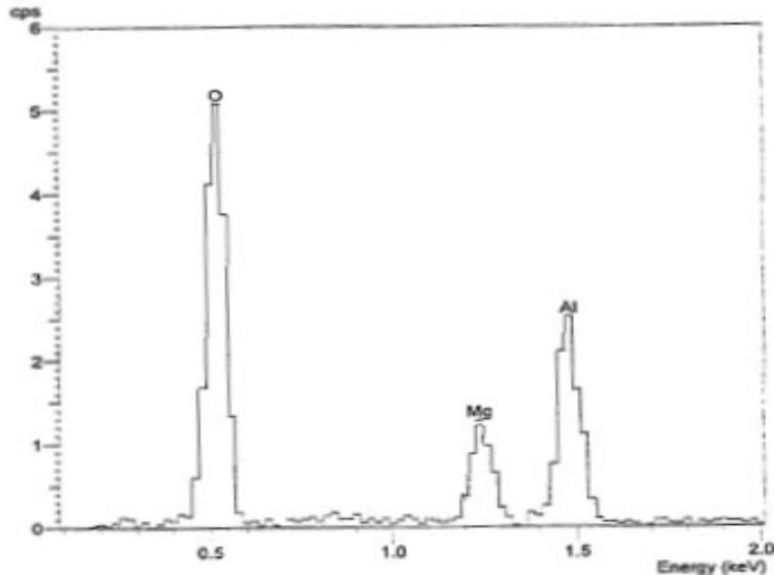
**Figure 5: EDS analysis of heat treated 6061/SiC metal matrix composite (SiC particle size = 10μm and volume fraction = 30%)**
