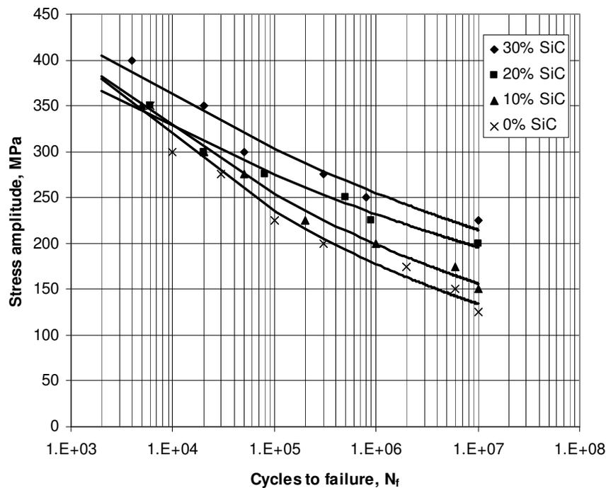
**Figure 10: S-N curves of heat treated 6061/SiC composites and 6061 matrix alloy**
