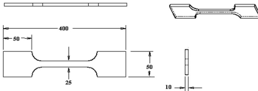
**Figure 2: Tensile specimen, all dimensions are in mm**
