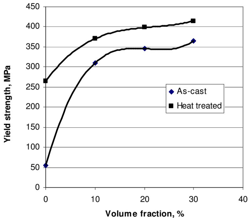
**Figure 6: Variation of the yield strength with the volume fraction of SiC particles**
