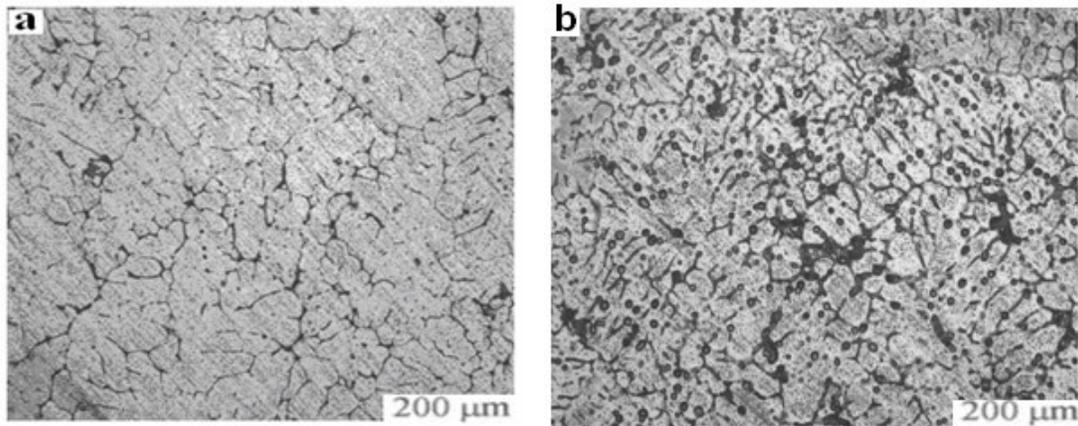
**Figure 4: Microstructure of (a) as-cast 6061/SiC<sub>p</sub> metal matrix composite and (b) heat treated 6061/SiC<sub>p</sub> metal matrix composite (volume fraction = 20%).**
