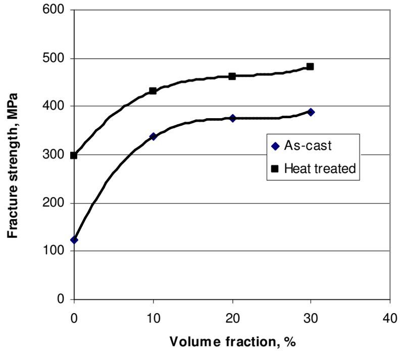
Figure 8: Variation of the fracture strength with the volume fraction of SiC particles
