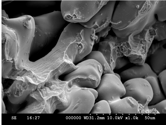
Figure 9: SEM of fracture surface of Al_2O_3 /Al6061 metal matrix composite, 1000X
