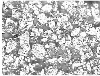
**Figure 2:** Microphotograph of Al-10%FA-300MP at 400X
