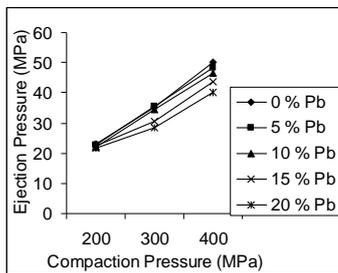
**Figure 4:** Effect of Compaction Pressure on Ejection Pressure.
