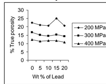
**Figure 9:** Effect of Lead content on % True Porosity.
