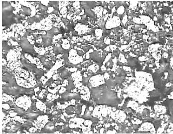
**Figure 1:** Microphotograph of Al-10%FA-200MP at 400X
