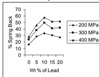
**Figure 11:** Effect of Lead content on % Spring Back.
