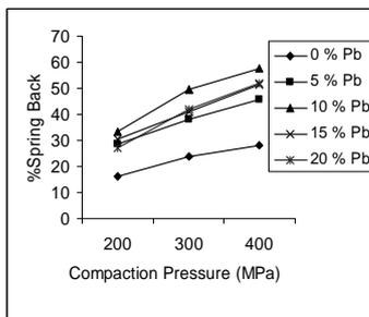
**Figure 10:** Effect of Compaction Pressure on % Spring Back..
