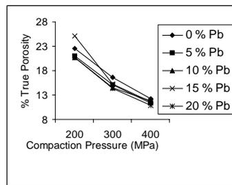
**Figure 8:** Effect of Compaction Pressure on % True Porosity.
