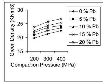
**Figure 6:** Effect of Compaction Pressure on Green Density
