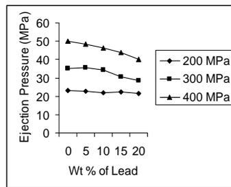
**Figure 5:** Effect of Lead content on Ejection Pressure.
