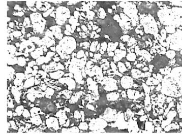
**Figure 3:** Microphotograph of Al-10%FA-400MP at 400X
