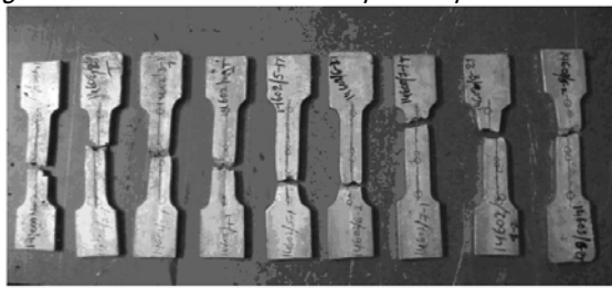
Fig. 3. Tested tensile Al/SiC composite specimens
