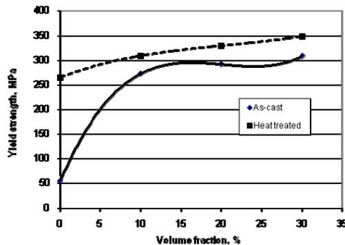
**Figure 6:** Variation of yield strength with volume fraction of  $\text{Al}_2\text{O}_3$  (a) As-cast, and (b) heat-treated.
