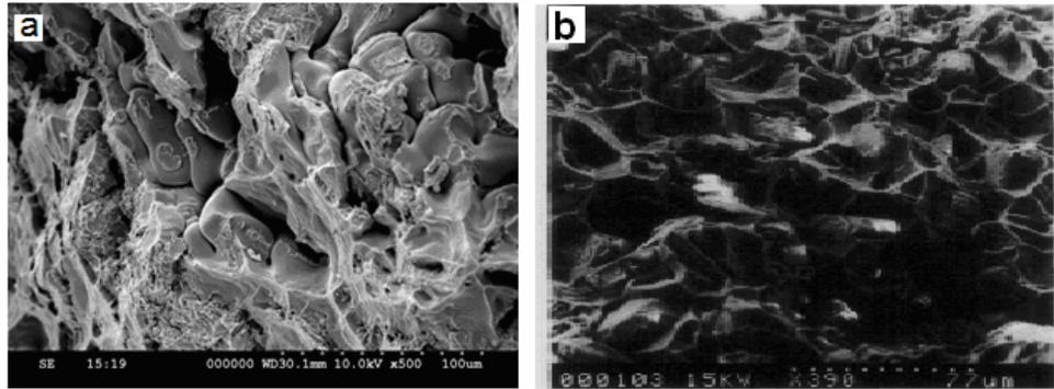
**Figure 12:** SEM tensile fracture surface of 6061/ 30%  $\text{Al}_2\text{O}_3$  composite (a) present work and (b) previous work (after Shakeri and Wang [23]).
