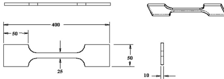
**Figure 3:** Tensile specimen, all dimensions are in mm.
