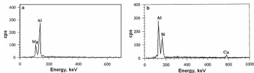
**Figure 5:** EDX spectrum shows the major elements that present in the interfacial reaction products. (a)  $\text{MgAl}_2\text{O}_4$  spinel or magnesium oxide ( $\text{MgO}$ ), and (b)  $\text{Al}_5\text{Cu}_2\text{Mg}_8\text{Si}_6$  or  $\text{Al}_4\text{CuMg}_5\text{Si}_4$
