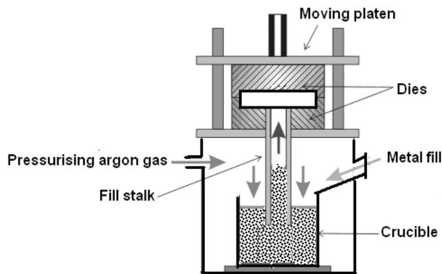
**Figure 1:** Low-pressure die casting process.
