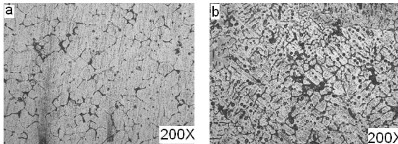
**Figure 4:** Microstructure of 6061/ $\text{Al}_2\text{O}_3$  composite (a) As-cast, and (b) heat-treated.
