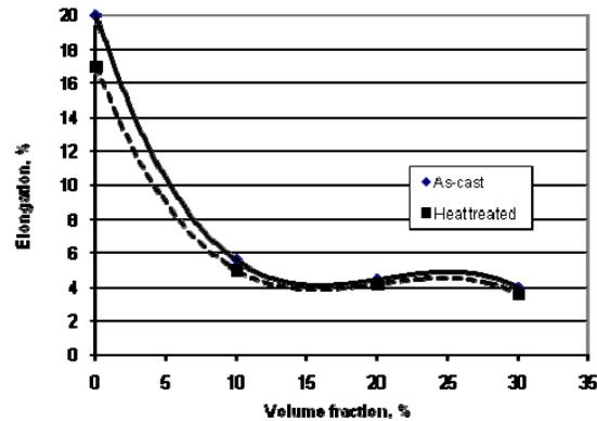
**Figure 10:** Variation of tensile elongation with volume fraction.
