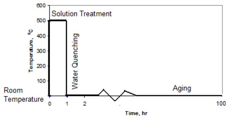
**Figure 2:** Heat treatment of 6061/Al<sub>2</sub>O<sub>3</sub> composite.
