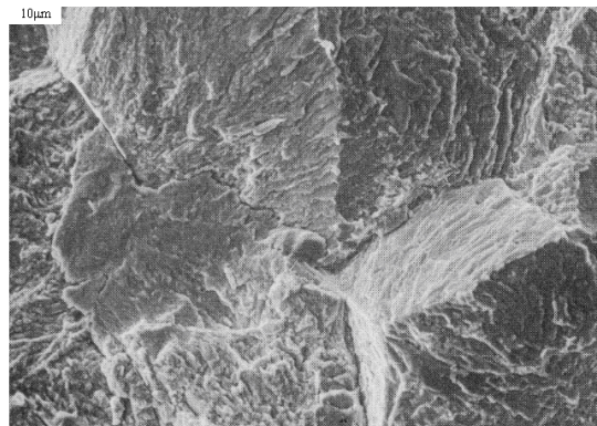
Figure 6. Intergranular fracture surface of a specimen containing a proeutectoid carbide network prior to austenitizing at 800°C.
