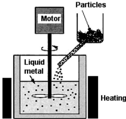
Figure 1: Charge preparation in the stir casting process
