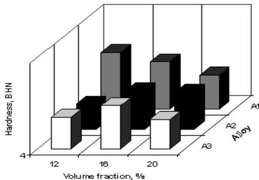
Figure 5: Effect of interaction between matrix alloy and volume fraction on harness of Al-alloy/Al<sub>2</sub>O<sub>3</sub> composite
