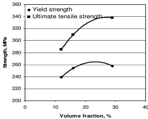
Figure 9: Influence of volume fraction on the yield strength of Al-alloy/Al<sub>2</sub>O<sub>3</sub> composite
