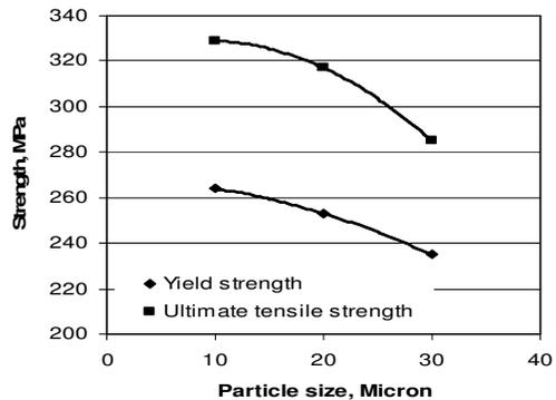
Figure 11: Influence of particle size on the yield and ultimate tensile strengths of Al-alloy/Al<sub>2</sub>O<sub>3</sub> composite
