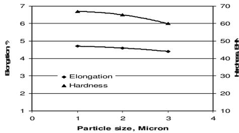
Figure 12: Influence of particle size on the ductility and hardness of Al-alloy/Al<sub>2</sub>O<sub>3</sub> composite
