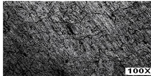
Figure 6: Microstructure of 6061/Al<sub>2</sub>O<sub>3</sub> composite
