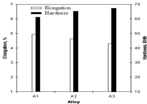
Figure 4: Influence of matrix alloy on the ductility and harness of Al-alloy/Al<sub>2</sub>O<sub>3</sub> composite
