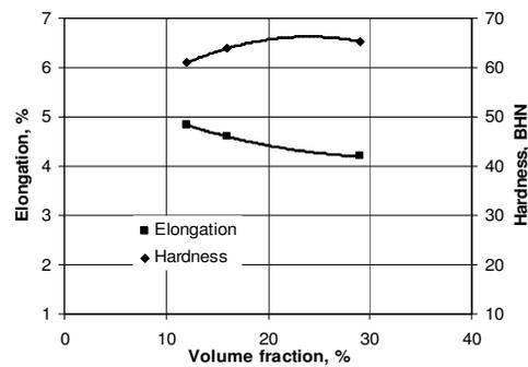
Figure 10: Influence of volume fraction on the ductility of Al-alloy/Al<sub>2</sub>O<sub>3</sub> composite
