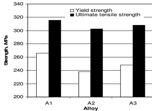
Figure 3: Influence of matrix alloy on the yield and ultimate tensile strengths of Al-alloy/Al<sub>2</sub>O<sub>3</sub> composite
