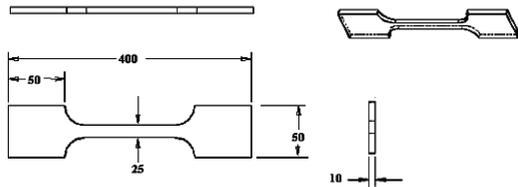
Figure 2: Tensile specimen, all dimensions are in mm
