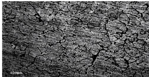
Figure 8: Microstructure of 7072/Al<sub>2</sub>O<sub>3</sub> composite
