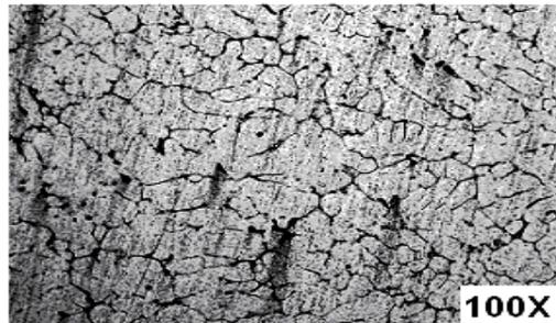
Figure 7: Microstructure of 6063/Al<sub>2</sub>O<sub>3</sub> composite
