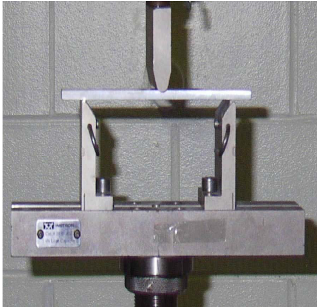
Figure 4. Three-point bend testing
