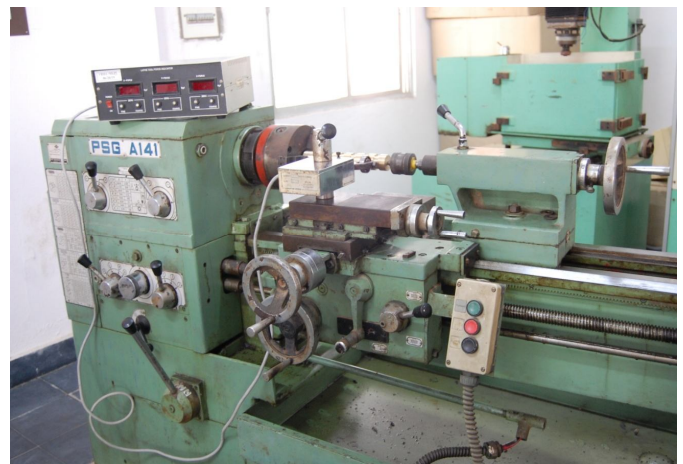
Fig. 11. Photograph of experimental set up of Roller burnishing process with brass work piece on PSG lathe.
