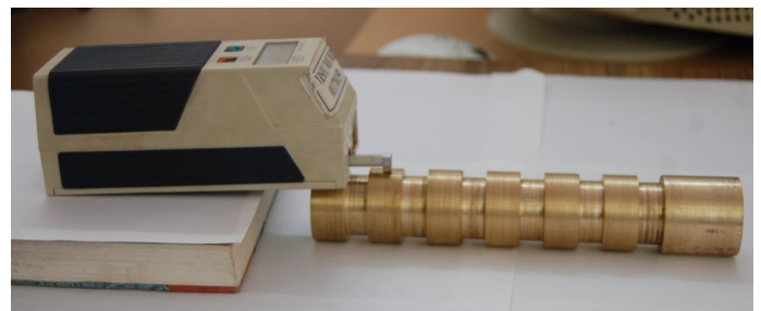
Fig.13.Measurement of Surface Roughness on Brass Specimen.
