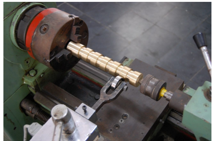
Fig12 Photograph showing close up view of brass work piece with roller burnishing tool on lathe.
